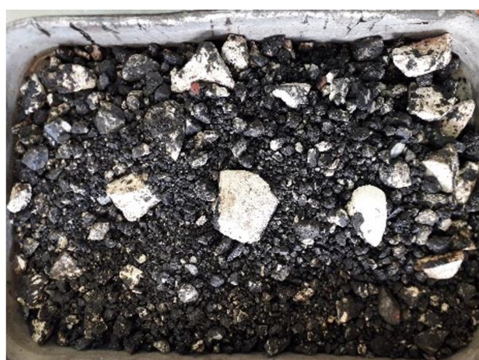
Sample of milled material for lab testing
