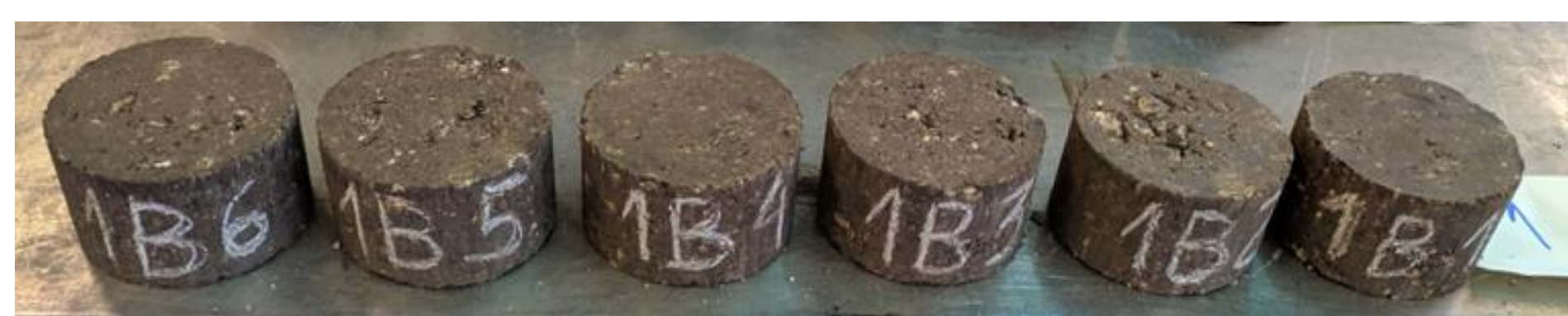
Specimens of cold recycled material with foamed bitumen produced in the laboratory
