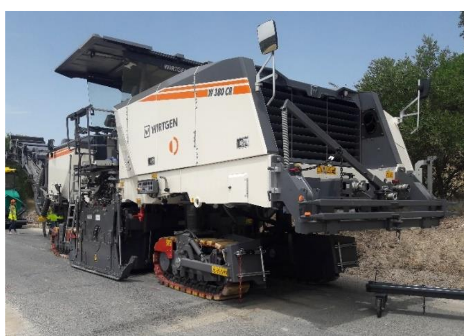
Recycler used for full-depth reclamation and addition of foamed bitumen
